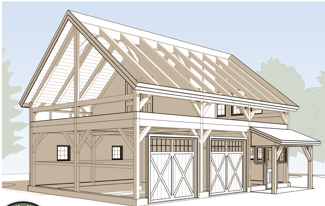
INTERIOR FRAME VIEW
